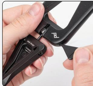
Insert the key in the **Tuning Access Hole**. Once engaged, tighten or loosen **Ballhead** to desired resistance, 1/8 turn at a time.
