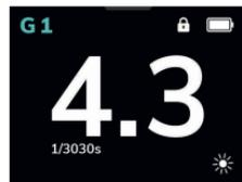
To activate the touch screen lock, press the ON button whilst powering on the unit for 9s. The lock symbol indicates that the touch screen is locked. To unlock switch the unit off and on again.
