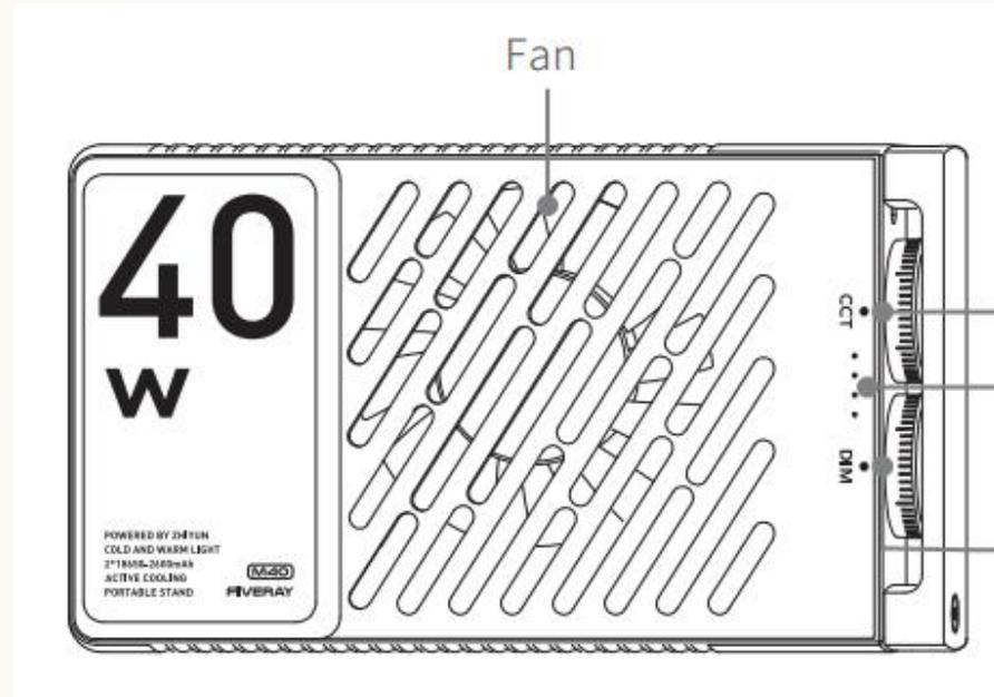
Adaptive fan inside M40 will adjust the cooling power according to different temperatures for more effective cooling.
