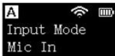
**Input Mode:** The input mode can be selected to Mic In or Line In. When the input mode is Mic In mode, the transmitter can be connected to the included lavalier microphone, or other microphones with a 3.5mm output. When the input mode is Line In mode, the receiver can be connected to line-level output devices. The system's default is "Mic In".
