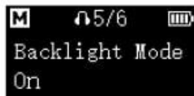
**Set Backlight:** Set backlight to Always On or On for 10, 30, or 60 seconds. Default is "On".
