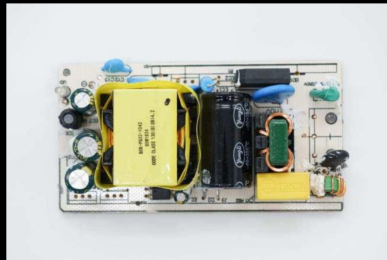
Multiple transformers and capacitors occupy more than half of the adapter's space
